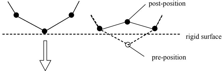
Figure 2. Pre-position and post-position of elastic collision in the constraint method.
