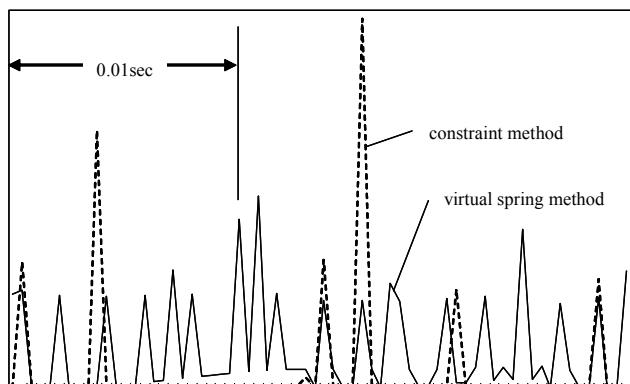
Figure 3. Feedback force generated by two kinds of collision algorithms.
