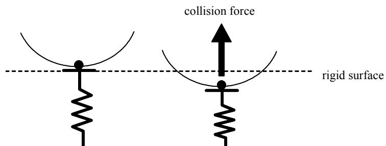
Figure 1. Collision force in the virtual spring method. The magnitude of collision force is proportionally increased according to the depth of vertex penetration.
